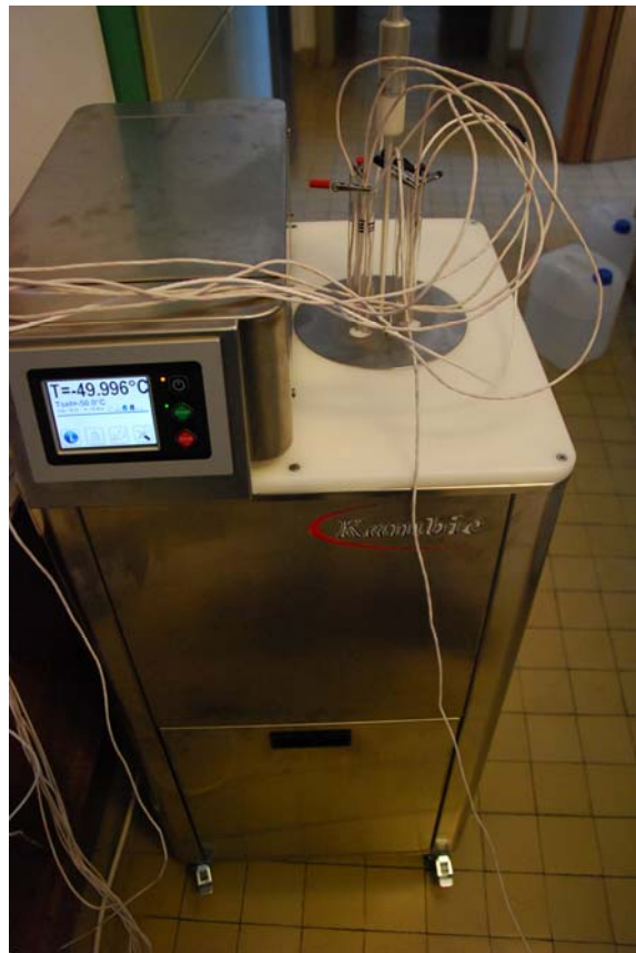
Figure 1: Kambič OB 7/2 ULT methanol bath with one reference thermometer and several PRTs under calibration
