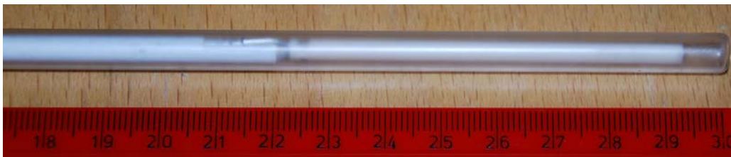
Figure 2: Used SPRT sensor
